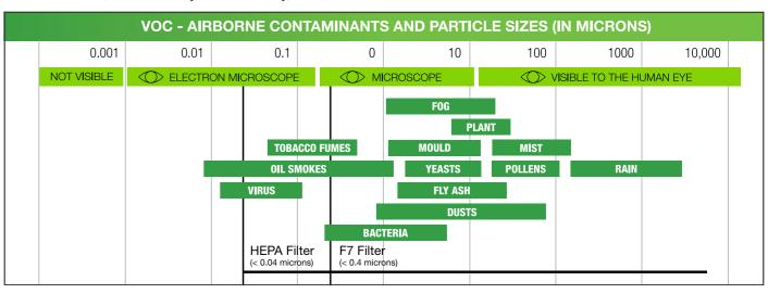
All centralised SmartVent systems feature high grade F7 filters that capture up to 90% of 0.4 microns particles such as fine pollens, dusts and allergen from the air making the air cleaner to breathe. High quality HEPA filters are also available for asthma and allergy sufferers.
